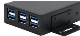
Mounting the Wall Mounting Bracket with four screws on each side
